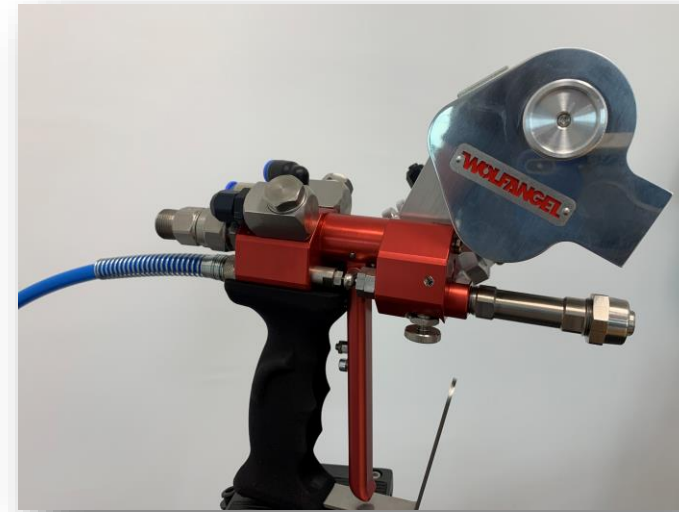
ergo.gun IC chopper gun internal mix with cutter SWII
