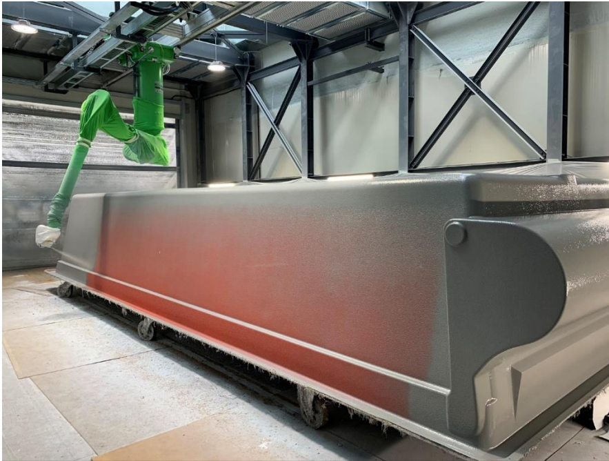
The robot can coat the complete component while hanging. Photos: Wolfangel/CMA
