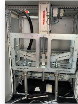
iJect touch EP Pumpenkombination P70/P40
