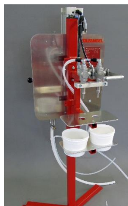
Outlets for resin and catalyst
