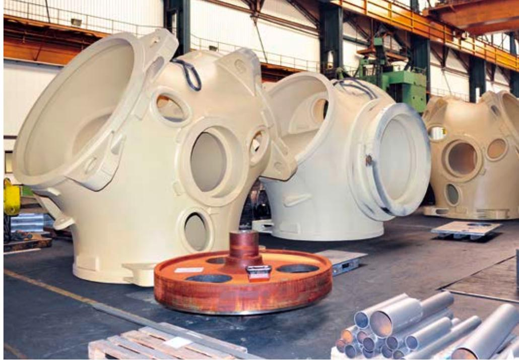
Rotor hub in the machining shop
