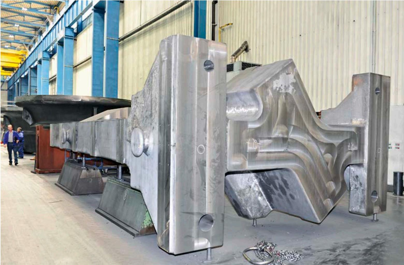
Press frame for a forging press in the machine shop
