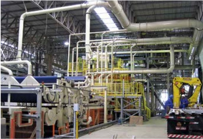
Forming line with pre-press and vapor exhaust
