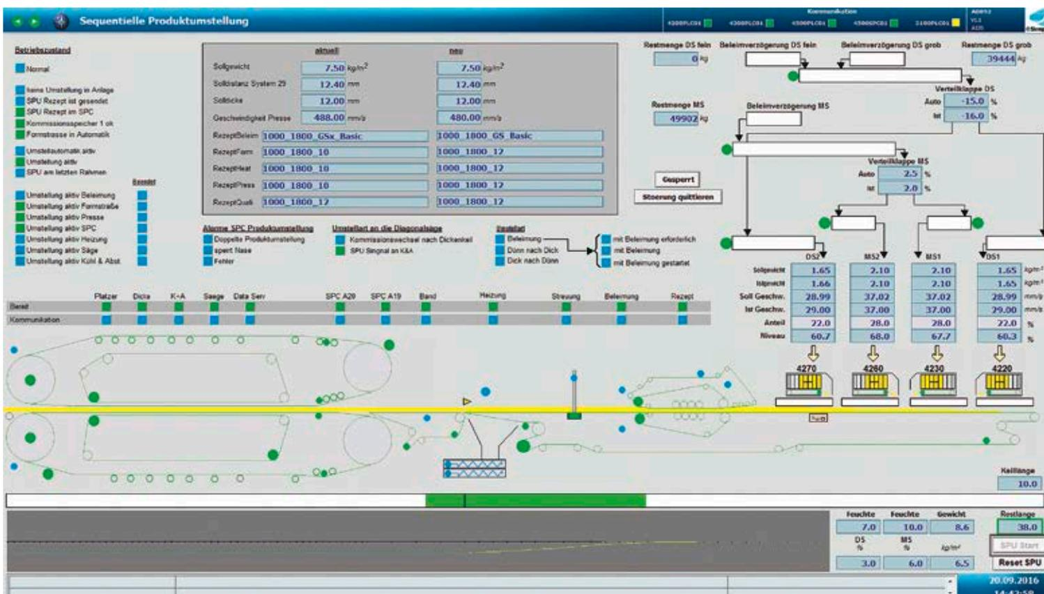
Visualization: The continuous green bar (at the bottom of the picture) represents the transitional wedge and illustrates the change in the weight
