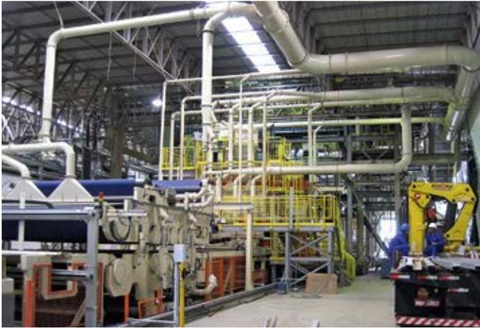
Forming line with pre-press and vapor exhaust
