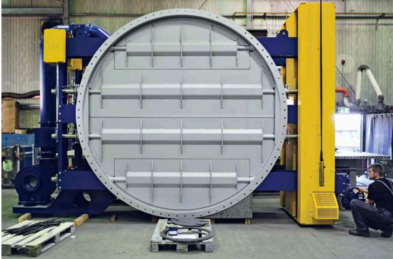
Man safe damper combination NW 3150 with sealing gas fan and pneumatic connections
