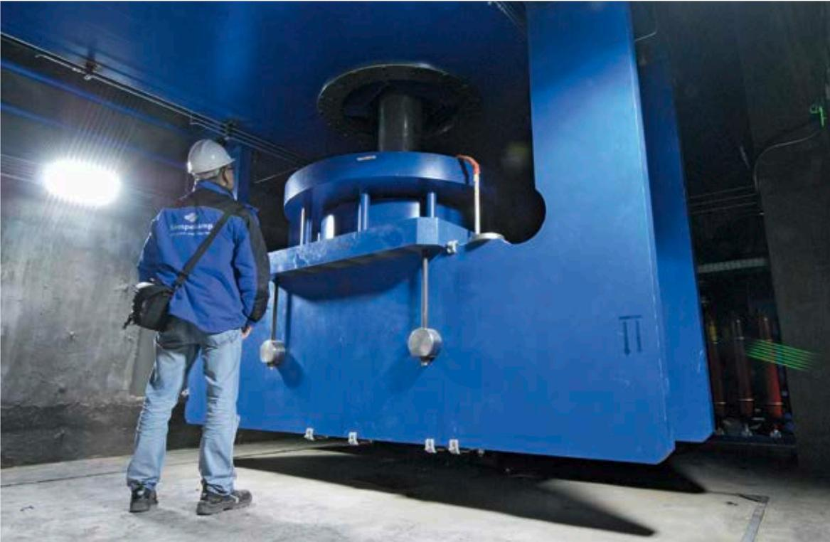
External ejector installed beneath the floor
