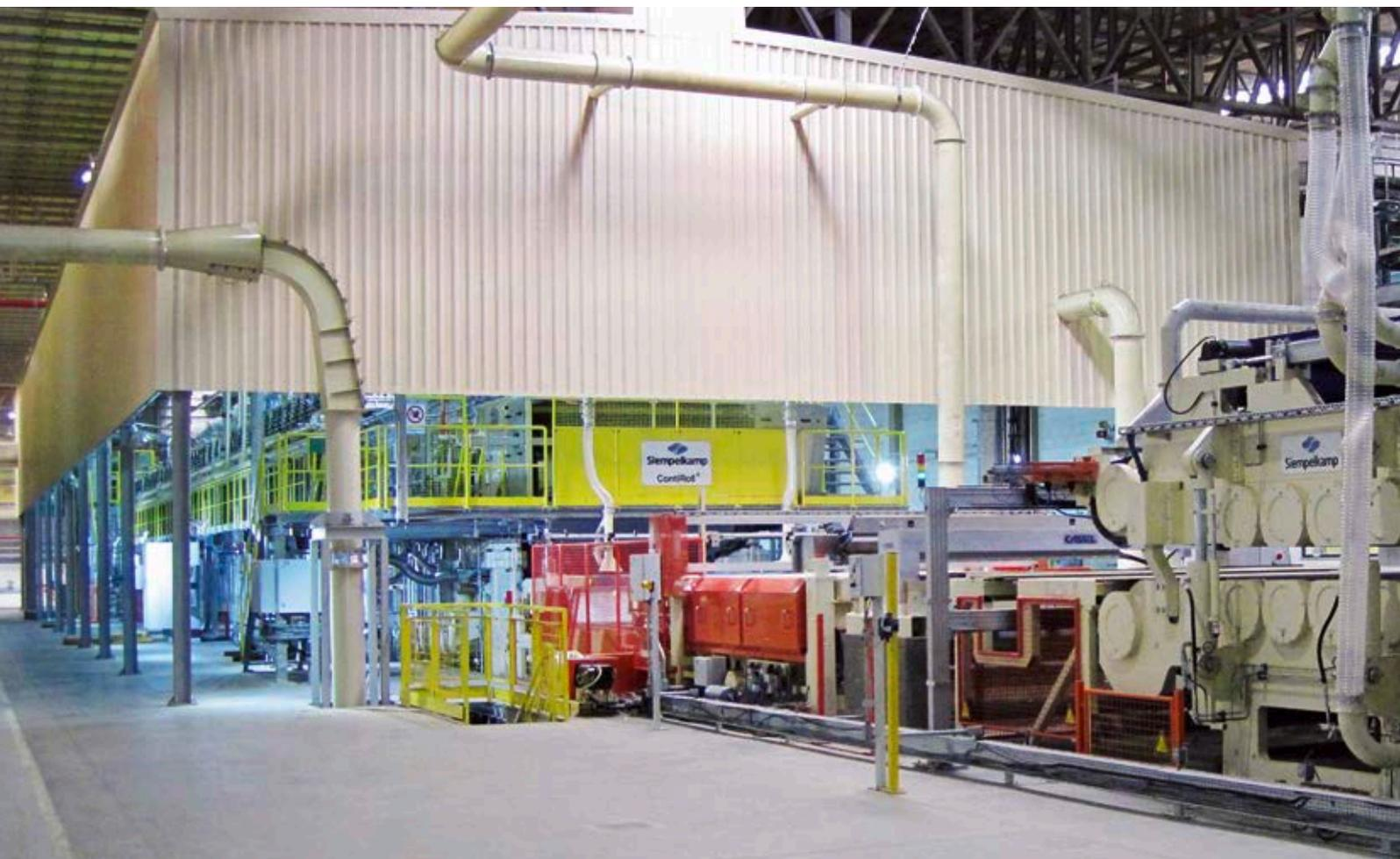
press and the company's second plant at the Curitiba location. With the existing ContiRoll® line the customer has been manufacturing MDF. The new line will add particleboard to the product range.
