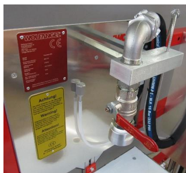
Outlets for resin and catalyst
